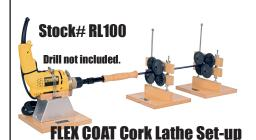
Set-up includes motor stand with motor clamps and 2 sets of roller supports. Adapts to almost any hand drill. Sturdy, commercial duty. This lathe is fantastic for shaping and reaming cork or foam grips. NOTE: We recommend a variable speed 0-2500RPM, 4.0 AMP hand drill.
