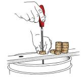
Using a rat tail file, a 1x4 board with a 1" hole and a 5 gallon bucket, ream the cork rings to a snug fit of the tapper of the blank.
